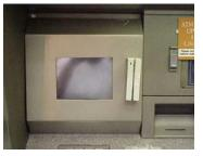
This photo shows an ATM at a metro bank location that has been altered to capture ATM and credit card info. This info is subsequently
